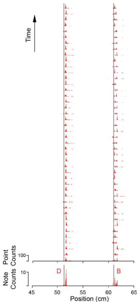
**Fig. 3** Two minutes of circuit data from a B-to-D trial from a single subject have been partitioned into one-note histograms. Time runs from *bottom* to *top*. The contact position at the peak of each single-note histogram was taken as a token for the pitch of that note in the sequence. This trial had 44 notes at each pitch. A composite histogram of peak values for these notes is shown at the *bottom*. The true B and D positions are shown as *vertical lines*
